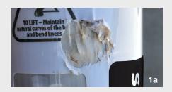
(1a) It is clear that the stand has been impacted. As you can see, the vinyl label has been damaged and delamination has occurred in the area. While the damaged specimen passed a WLL test, ANY STAND with this type of damage SHALL NOT be used.
